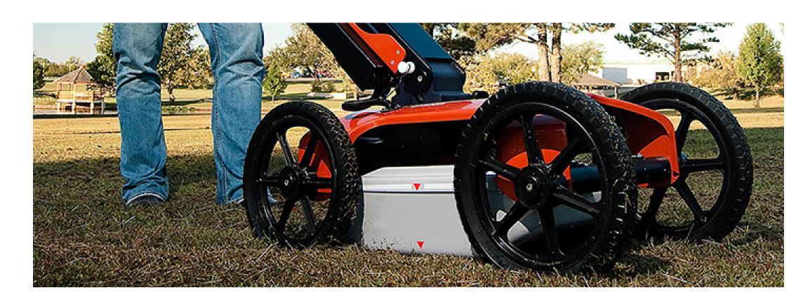
**Ground Penetrating Radar:** Ground Penetrating Radar (GPR) helps identify the location of underground utilities. A device that looks similar to a lawnmower, and is nondestructive to the soil, uses radio frequencies to detect objects below the ground's surface. Maps and images are created from the data.
