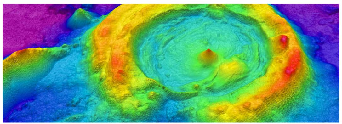
LiDAR: LiDAR (Light Detection and Ranging) uses laser pulses to measure the distance of an object to the source. The data points result in digital 3D maps for accurate design and engineering. LiDAR surveying crews use mobile (car or aerial vehicle) or static (tripod) equipment.
